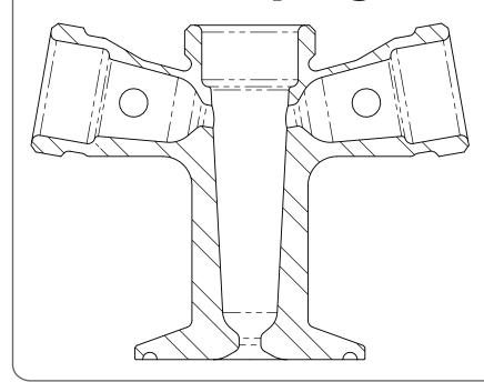
Pictured at left is a cutaway of our BSV Complex valve body. Machined out of one piece it is designed from the onset for maximum cleanability.
